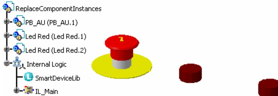
2. Select **Replace By Existing Device**
