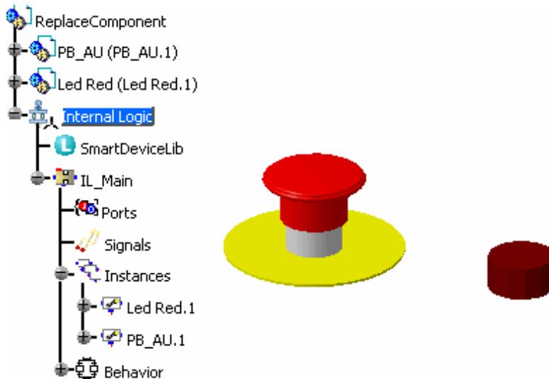
The internal logics of the devices LedRed and PB\_AU are instantiated in the root product.
