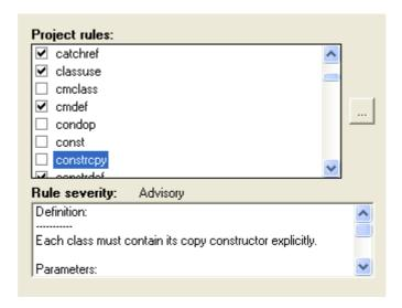
The last RuleChecker Settings dialog box allows to use some advanced features of the Logiscope RuleChecker module.
