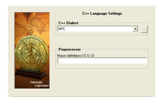
C++ Dialect: A dialect is used to specify parsing actions associated to some types, "keywords" according to the source code compiler specifics.
