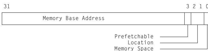
Figure 15. Base Address Register for Memory Access to I/O Local Address Space
