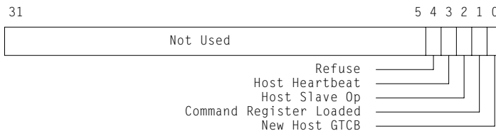
Figure 36. Adapter Interrupt Doorbell Register
