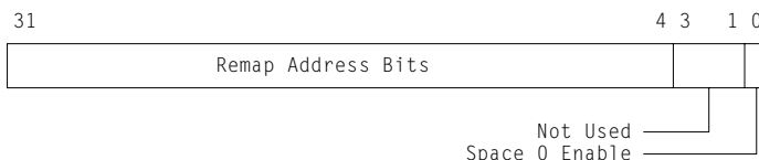
Figure 22. Local Address Space 0 Base Address (Remap) Register for PCI to Local Bus
