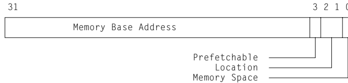
Figure 13. Base Address Register for Memory Access to Runtime Registers
