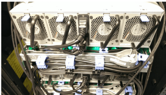
Figure 140. Power and SAS cable connections on the back of the enclosure
