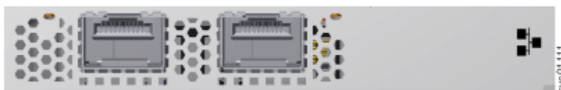
Figure 11. 25 Gbps Ethernet host interface adapter ports and LEDs (RoCE)
