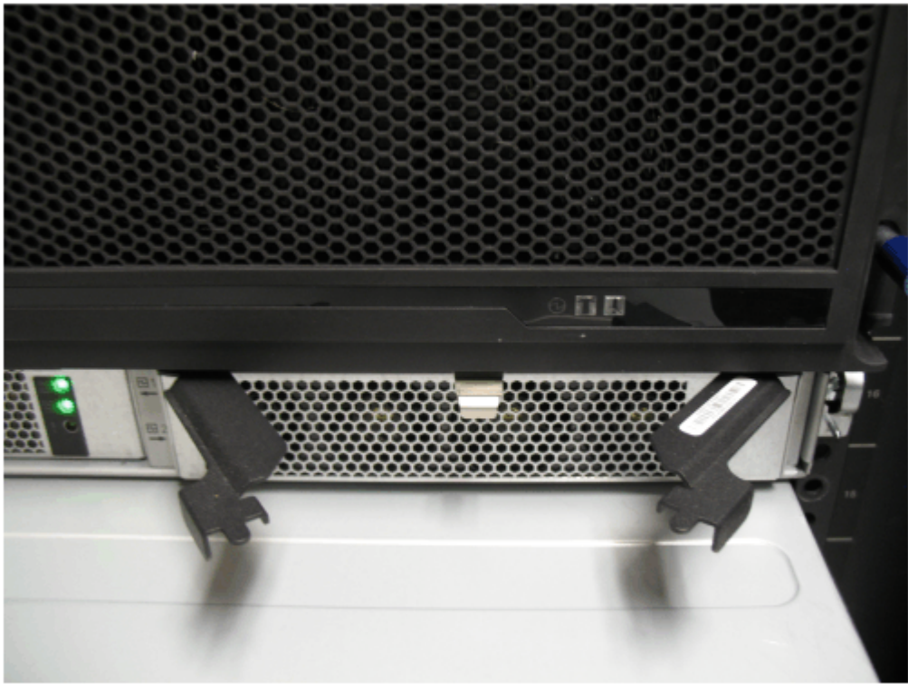
Figure 108. Releasing the power supply handles
