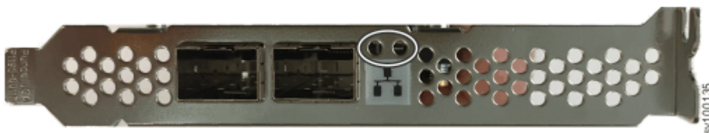
Figure 12. 25 Gbps Ethernet host interface adapter ports and LEDs (iWARP)
