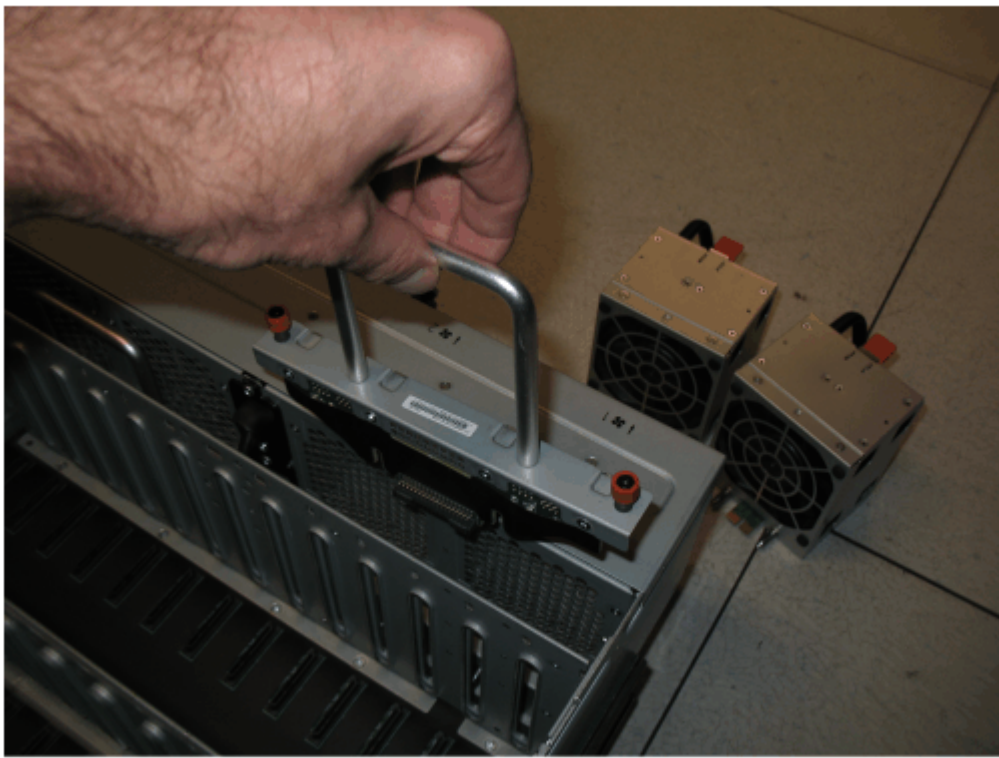
Figure 104. Insert the new FIB in the chassis
