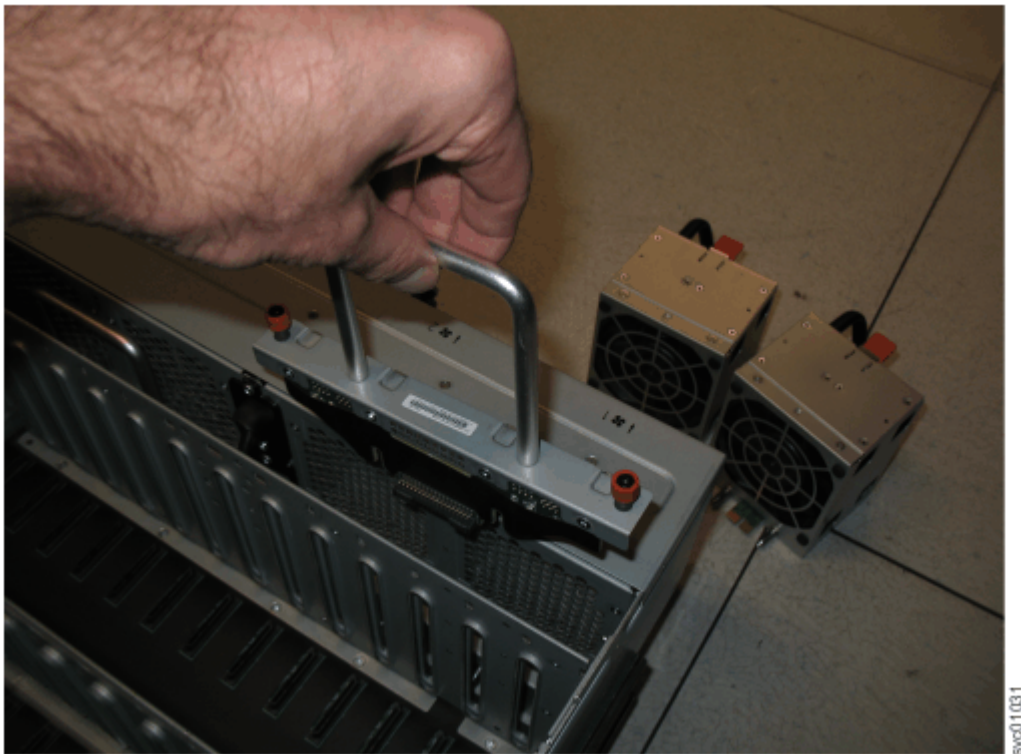
Figure 126. Remove the FIB from the chassis
