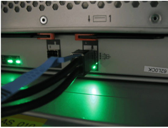
Figure 100. SAS cable correctly inserted into the SAS port
