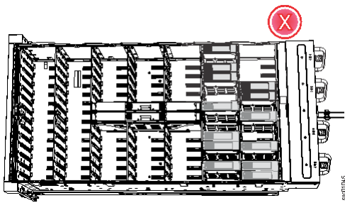
Figure 84. Incorrect drive installation
