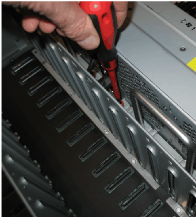
Figure 105. Secure the FIB to the drive board
