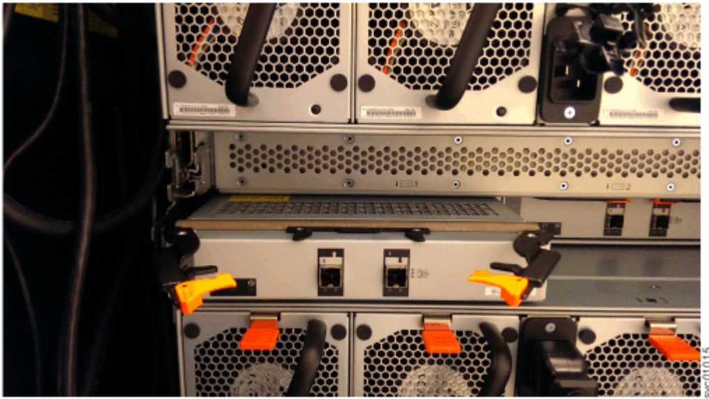
Figure 119. Removing the expansion canister
