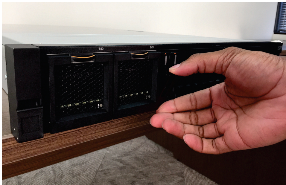
Figure 120. Operating the release handle on a 2145-SV1 boot drive
