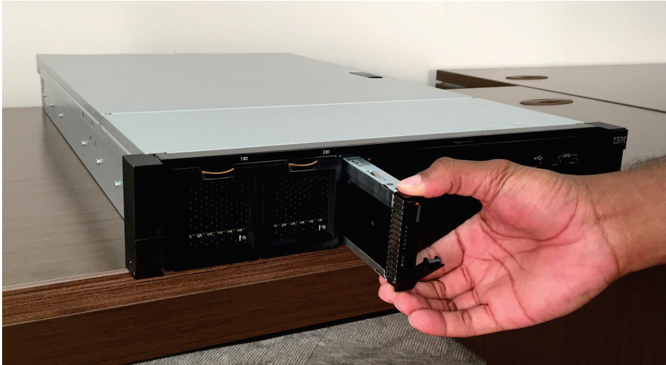
Figure 127. Aligning the 2145-SV1 boot drive
