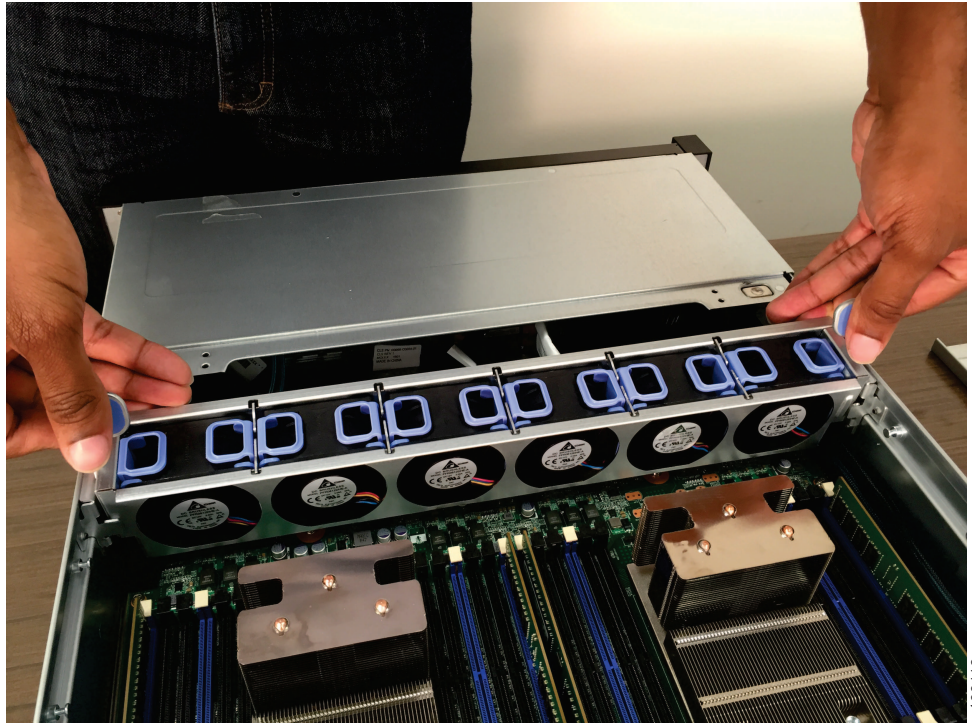
Figure 286. Replacing the fan bracket
