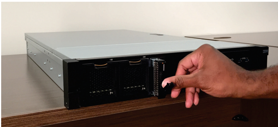
Figure 128. Replacing a 2145-SV1 boot drive
