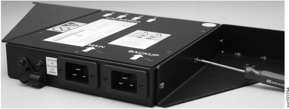
Figure 206. Attaching the mounting plates
