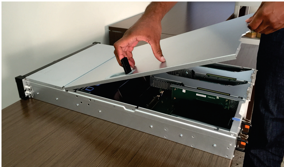
Figure 73. Removing the 2145-SV1 back cover
