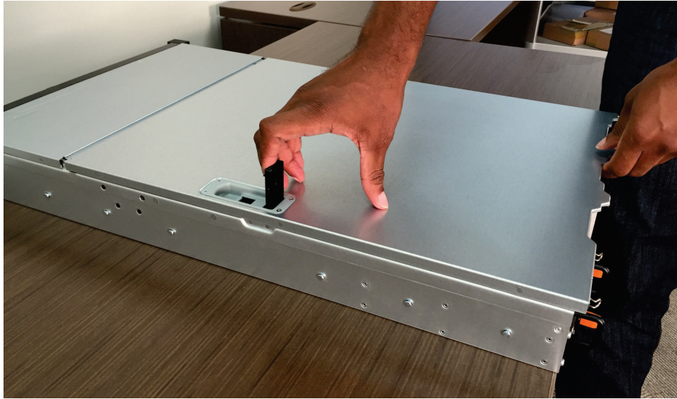
Figure 72. 2145-SV1 back cover release latch
