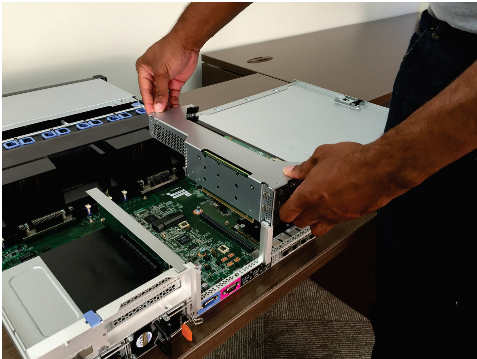
Figure 242. Aligning PCI riser card assembly 1
