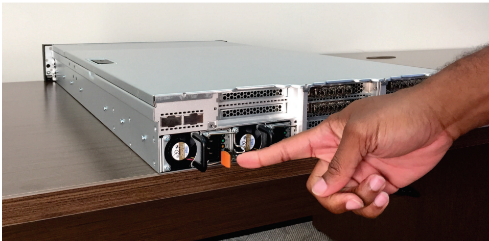
Figure 196. Release in the 2145-SV1 power supply
