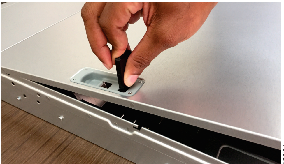
Figure 78. Replacing the 2145-SV1 back cover
