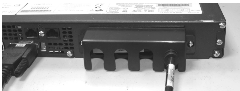
Figure 347. The 2145 UPS-1U cable retention bracket connected to the 2145 UPS-1U
