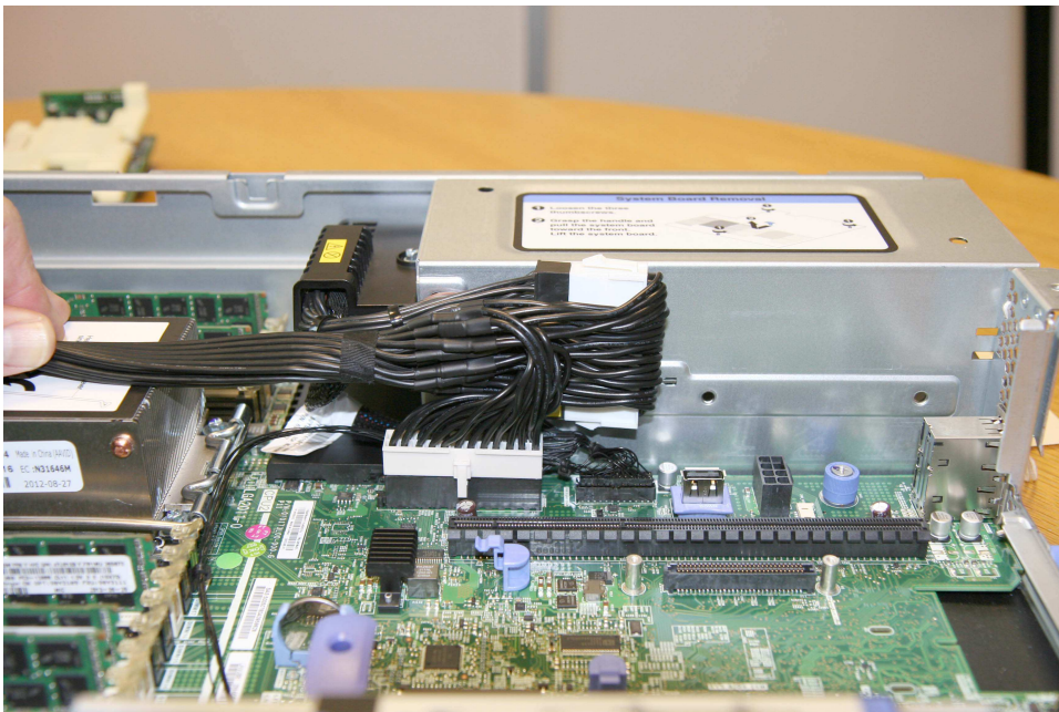
Figure 171. Power cable connection between the power supply unit and the system board
