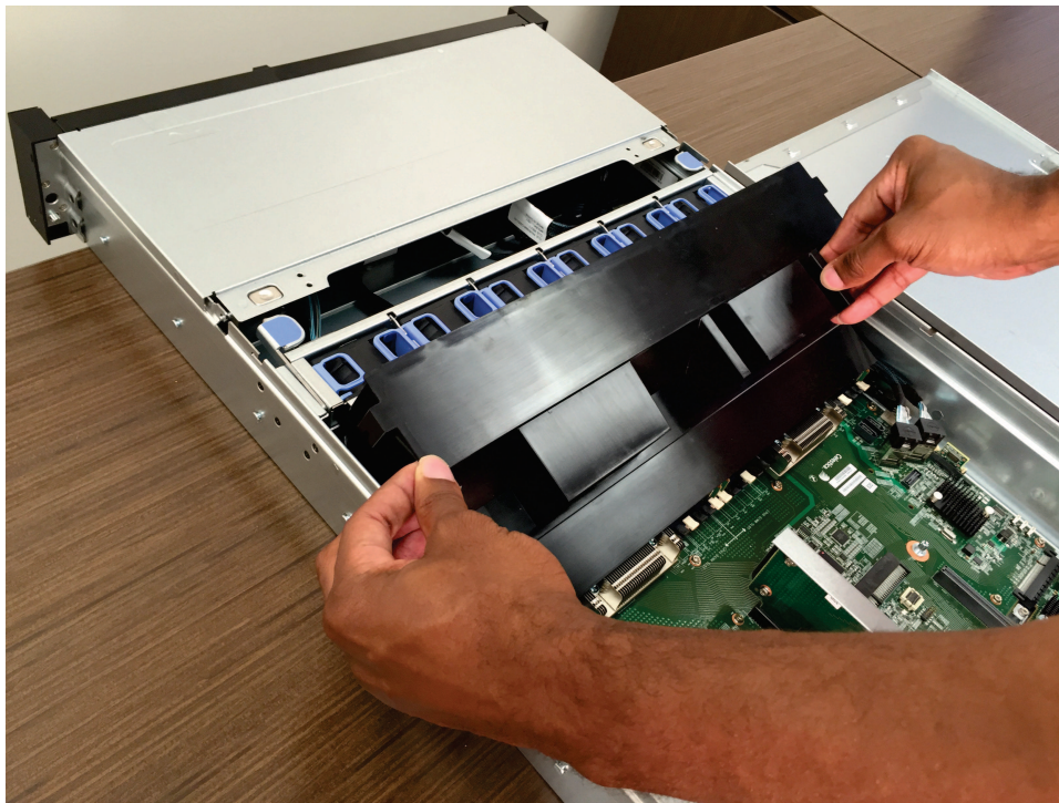
Figure 81. Removing the air baffle
