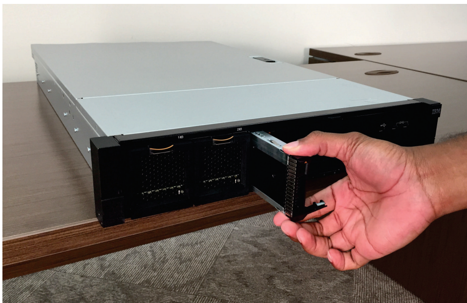
Figure 121. Removing a 2145-SV1 boot drive
