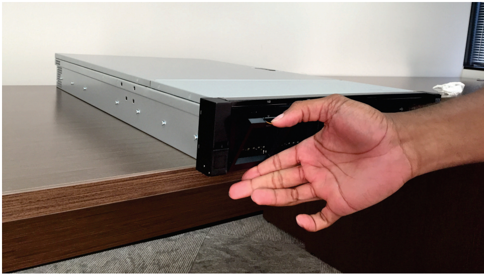
Figure 176. Release the battery module on the 2145-SV1 node
