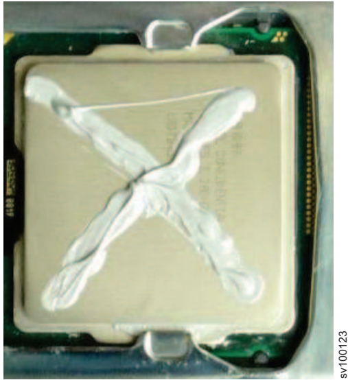
Figure 300. Applying thermal grease to the 2145-SV1 microprocessor
