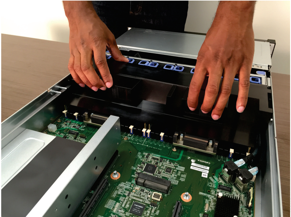
Figure 85. Replacing the air baffle
