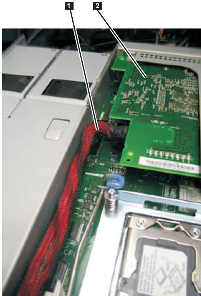
Figure 225. High-speed SAS adapter assembly and high-speed SAS cable in the SAN Volume Controller 2145-CG8 or 2145-CF8
