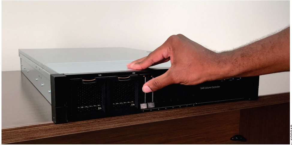
Figure 129. Closing the release handle on a 2145-SV1 boot drive
