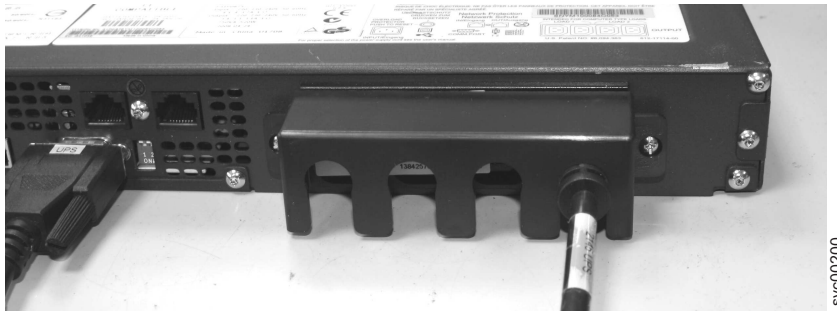
Figure 334. 2145 UPS-1U power cable-retention bracket
