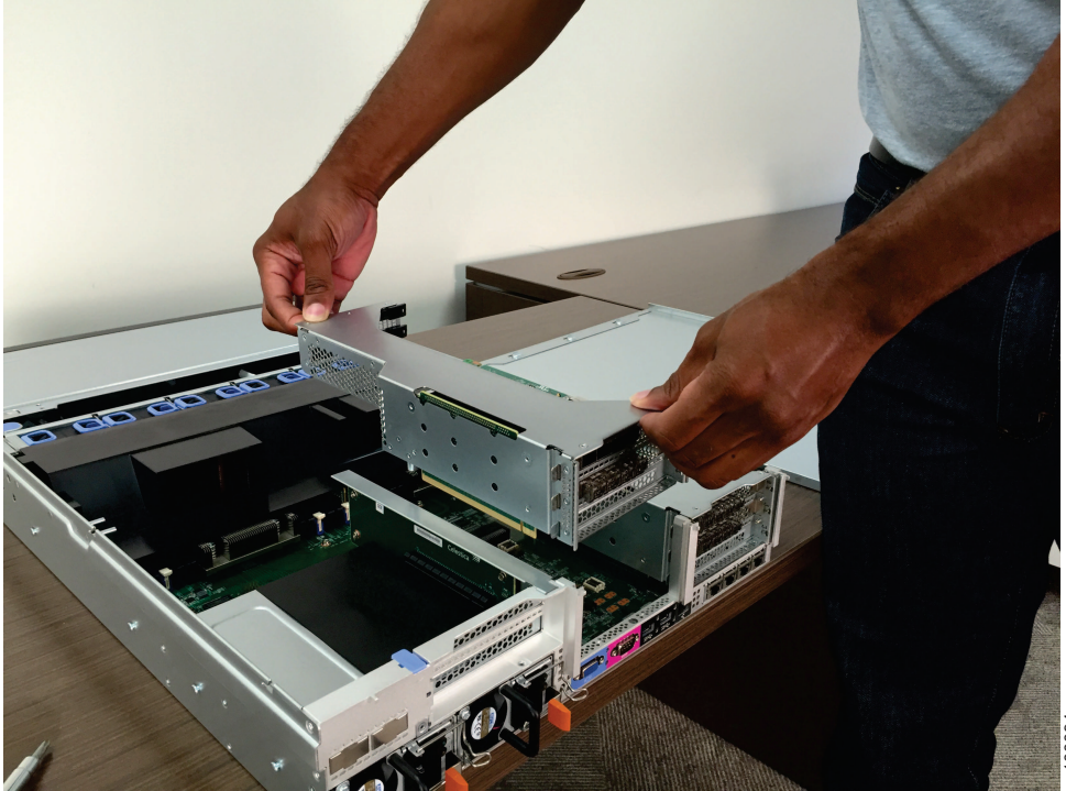
Figure 240. Grasping and removing PCI riser-card assembly 2
