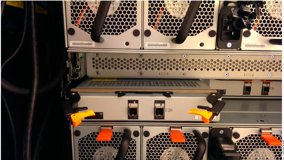
Figure 116. Removing the expansion canister
