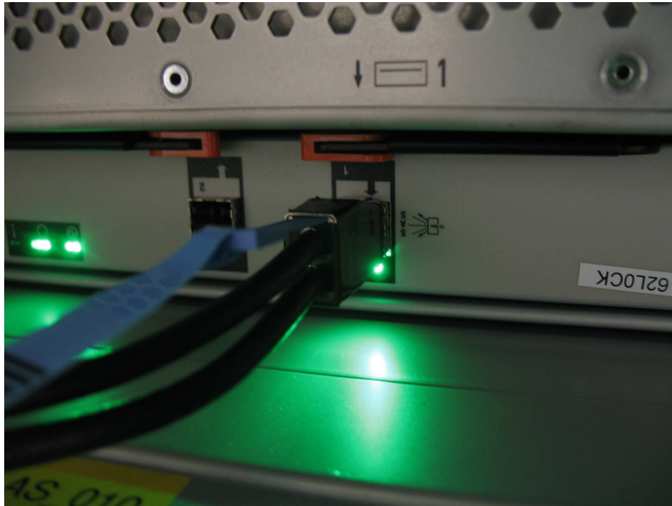
Figure 97. SAS cable correctly inserted into the SAS port
