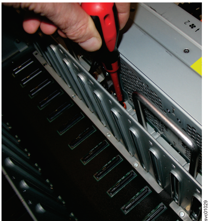
Figure 102. Secure the FIB to the drive board
