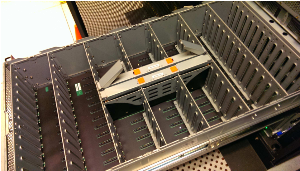
Figure 110. Location of secondary expander modules
