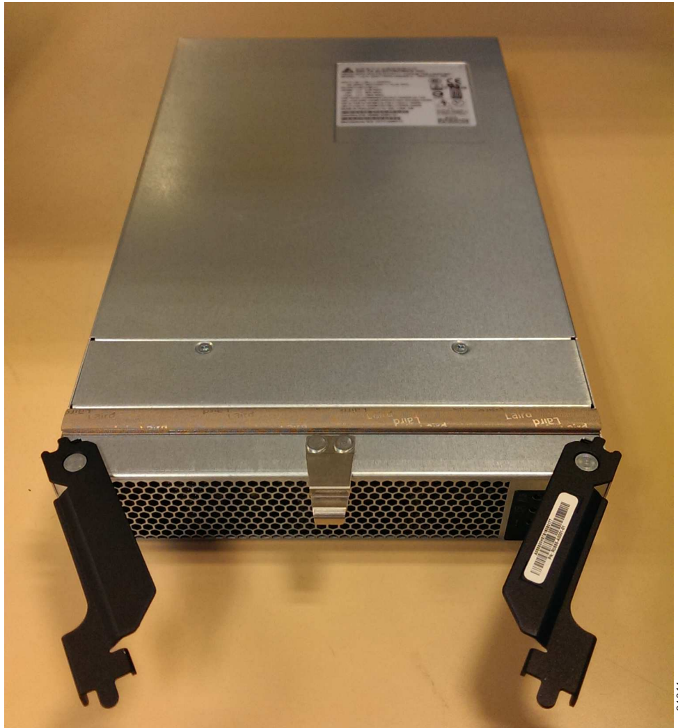
Figure 106. Removed power supply
