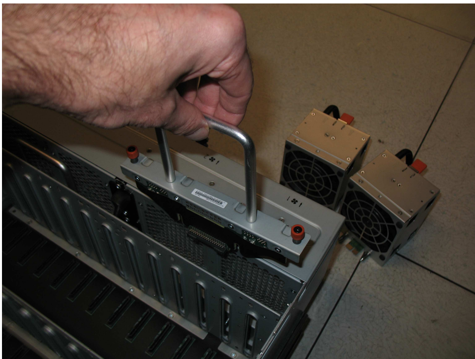
Figure 101. Insert the new FIB in the chassis
