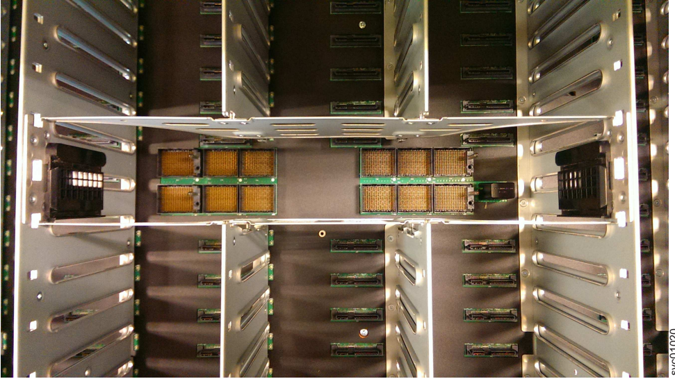
Figure 113. Secondary expander module connectors
