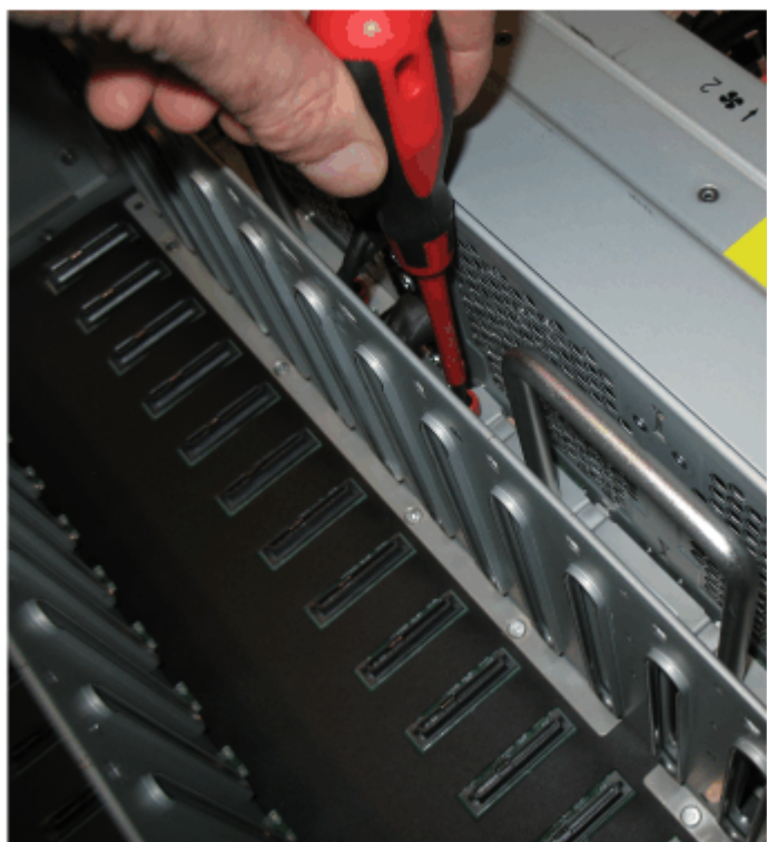
Figure 105. Secure the FIB to the drive board
