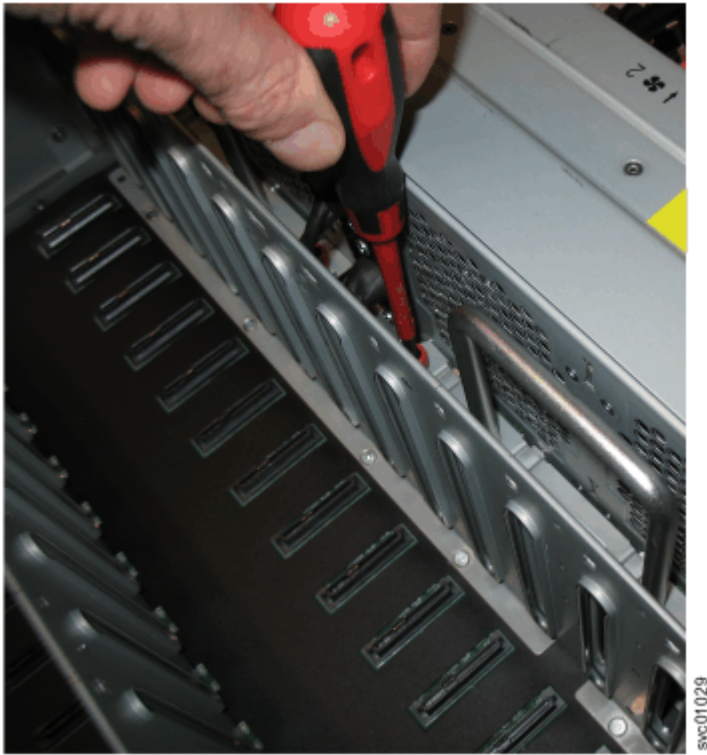
Figure 125. Loosen the FIB screws
