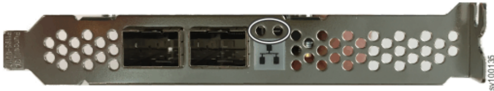
Figure 12. 25 Gbps Ethernet host interface adapter ports and LEDs (iWARP)
