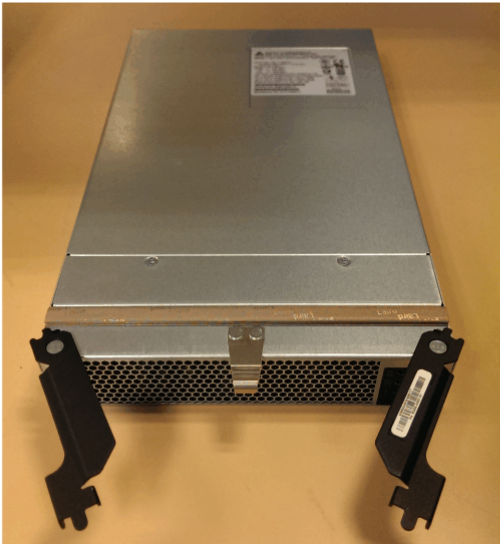
Figure 109. Removed power supply
