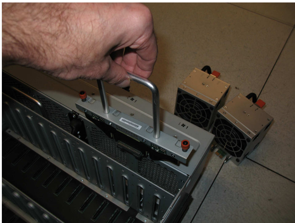
Figura 126. Remova a FIB do chassi
