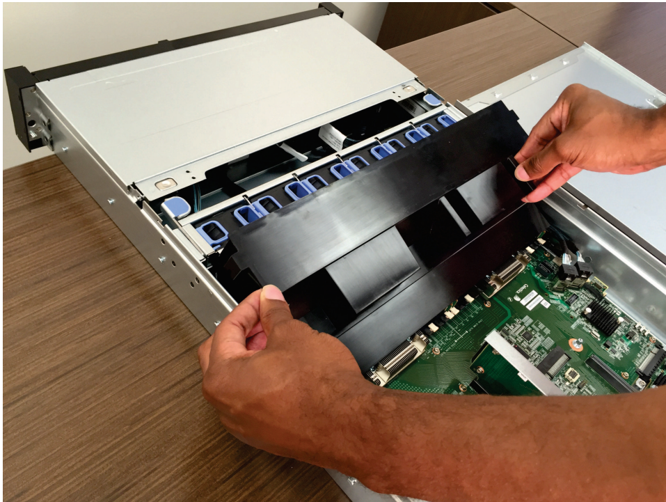
Figure 57. Removing the air baffle
