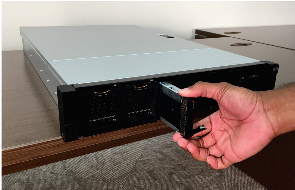
Figure 83. Removing a 2145-SV1 boot drive
