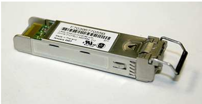
Figure 143. SFP transceiver
