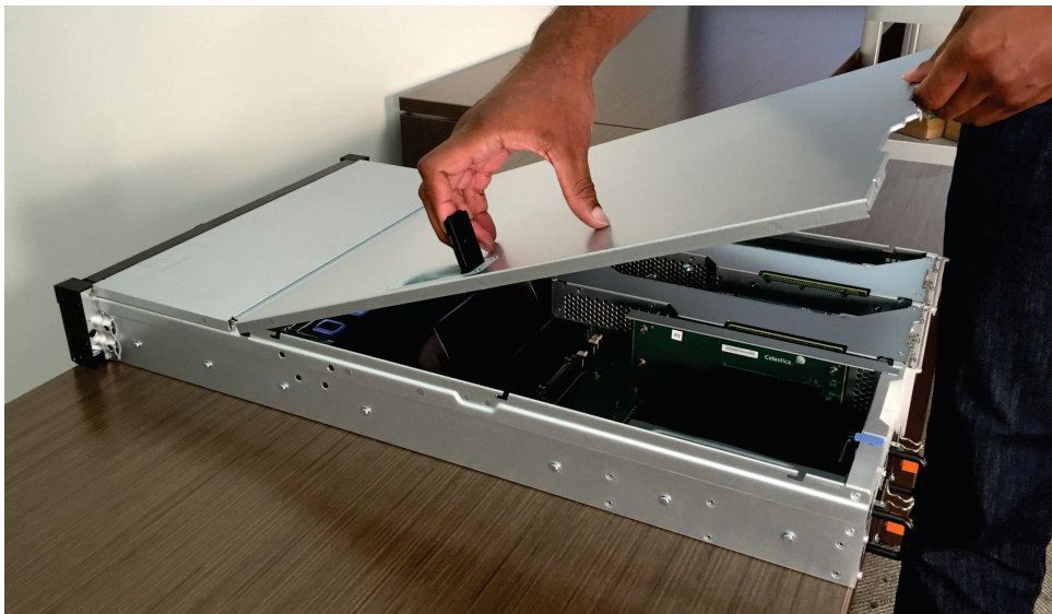
Figure 51. Removing the 2145-SV1 back cover
