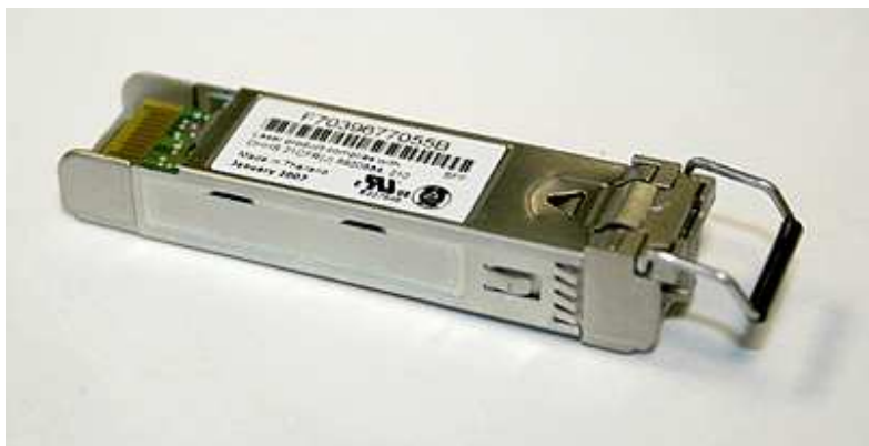
Figure 144. SFP transceiver
