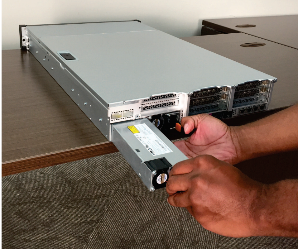
Figure 139. Replacing the 2145-SV1 power supply
