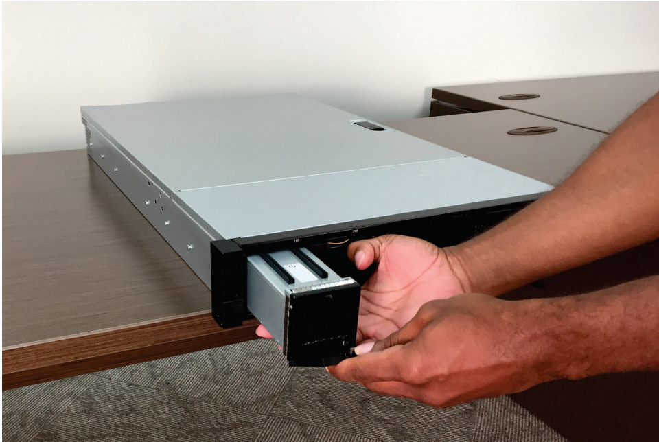
Figure 124. Replacing the battery in the 2145-SV1 node
