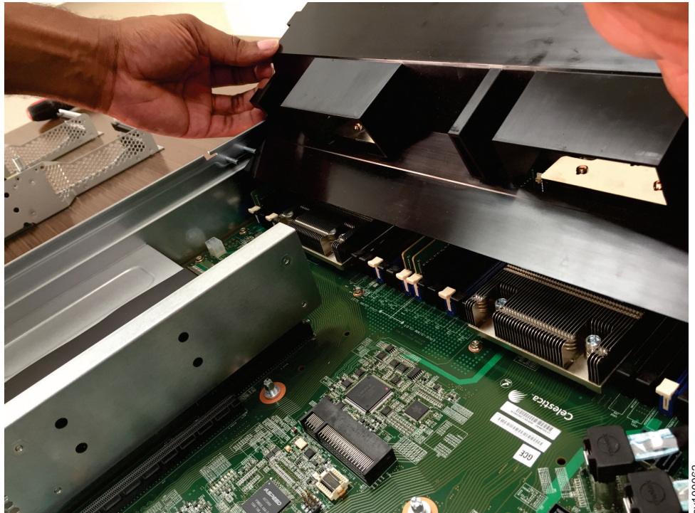
Figure 58. Removing the air baffle
