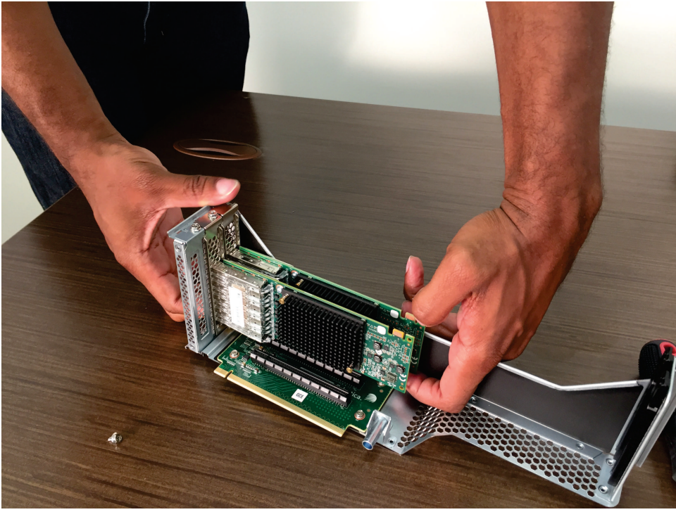
Figure 154. Unseating the adapter
