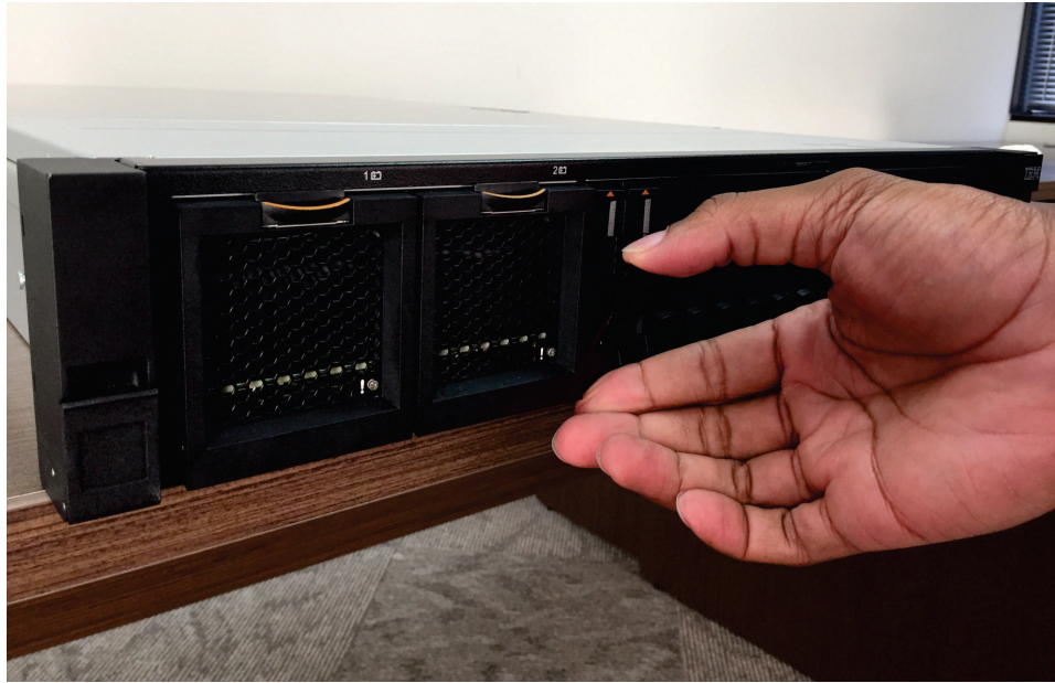
Figure 82. Operating the release handle on a 2145-SV1 boot drive
