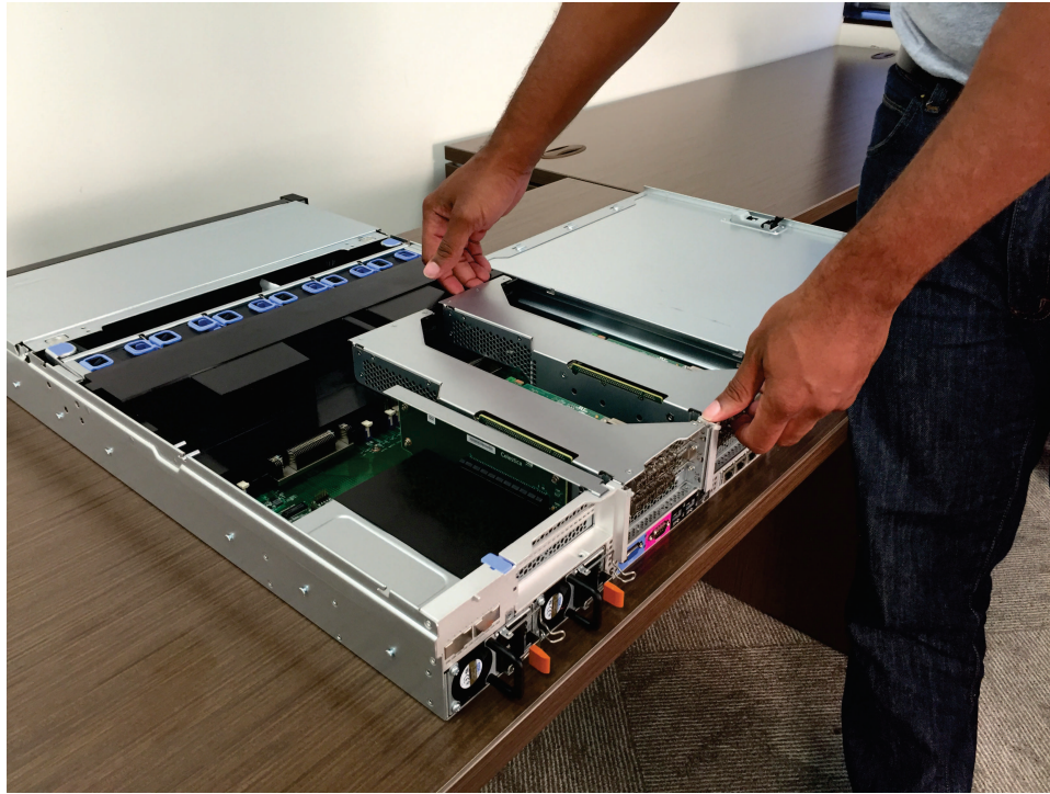
Figure 146. Grasping PCI riser-card assembly 1
