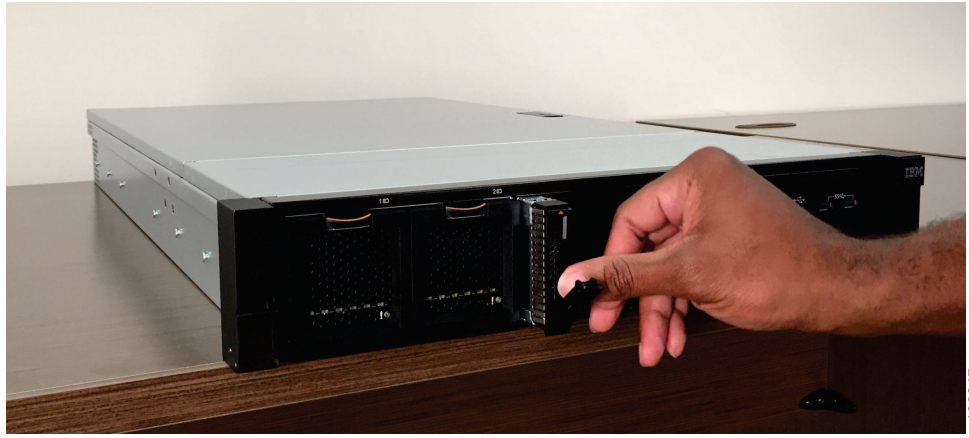
Figure 86. Replacing a 2145-SV1 boot drive
