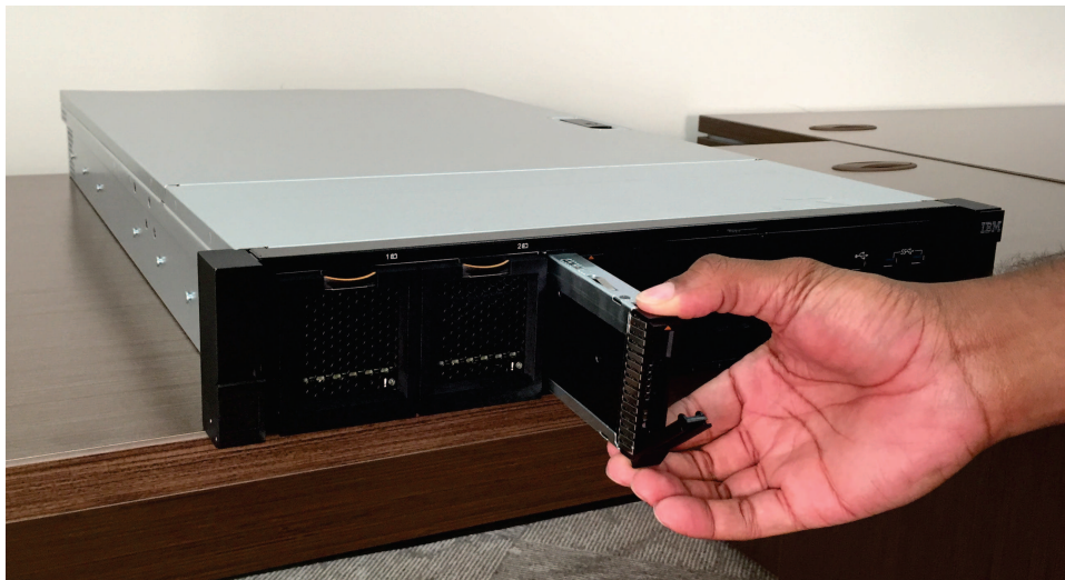
Figure 85. Aligning the 2145-SV1 boot drive
