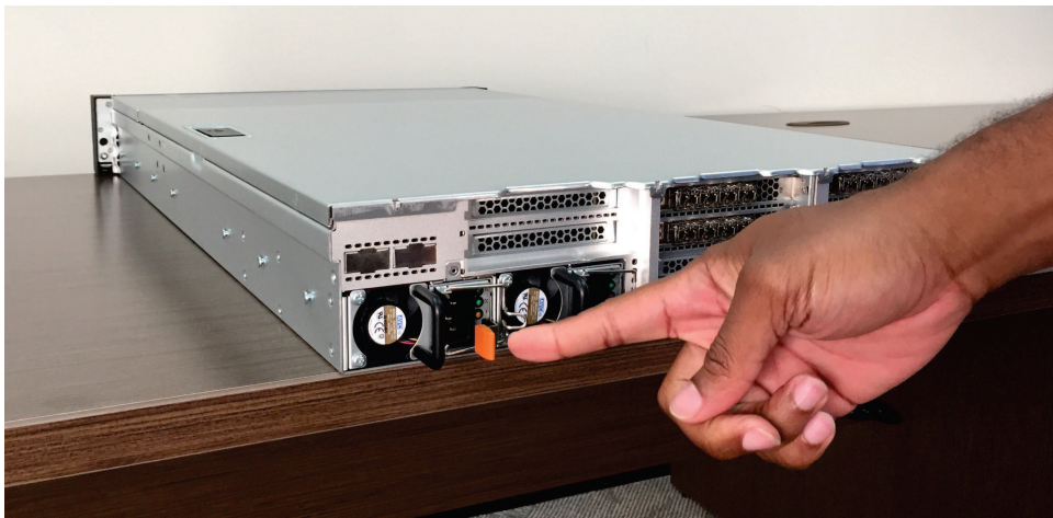
Figure 136. Release in the 2145-SV1 power supply
