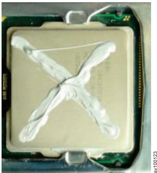
Figure 192. Applying thermal grease to the 2145-SV1 microprocessor
