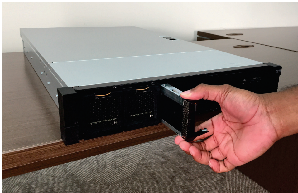
Figure 83. Removing a 2145-SV1 boot drive
