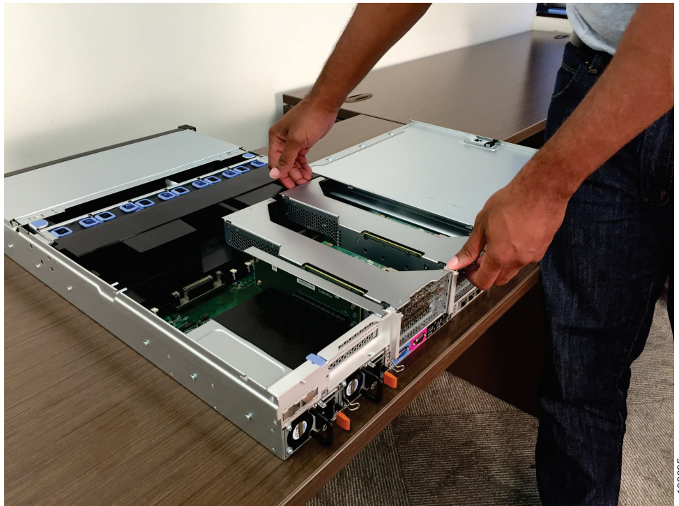
Figure 146. Grasping PCI riser-card assembly 1
