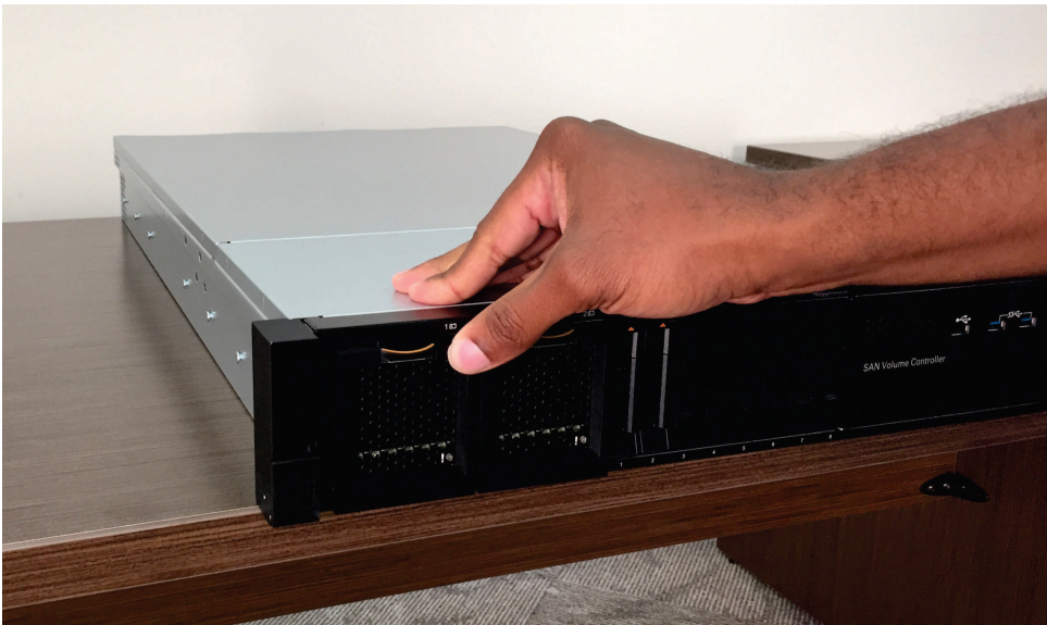
Figure 125. Closing the battery release handle
