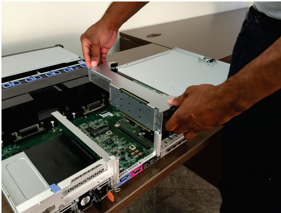
Figure 150. Aligning PCI riser card assembly 1
