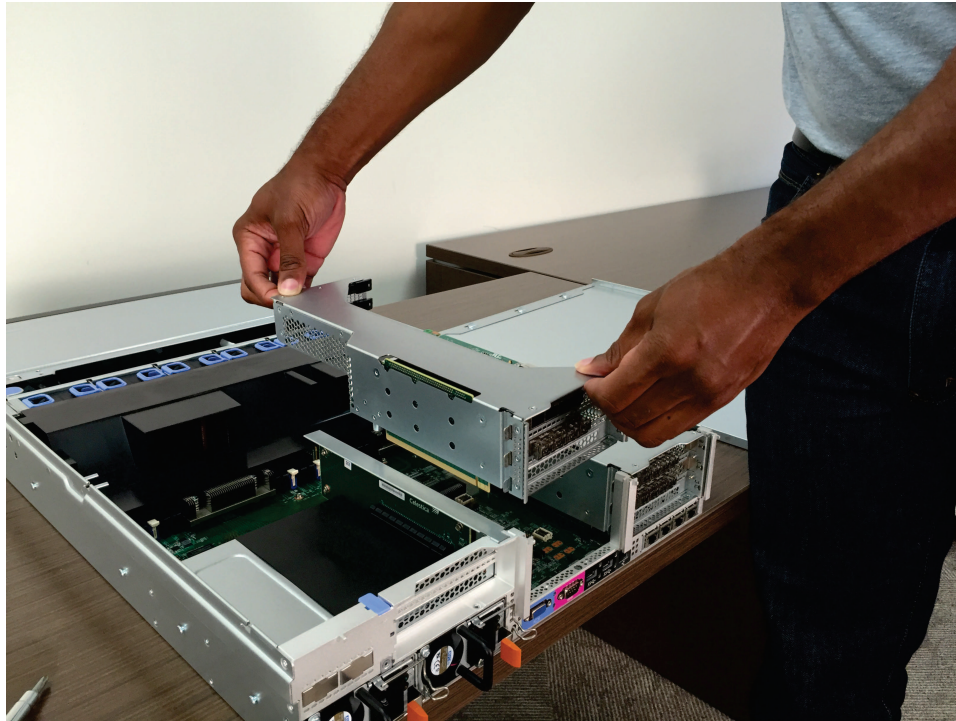
Figure 148. Grasping and removing PCI riser-card assembly 2
