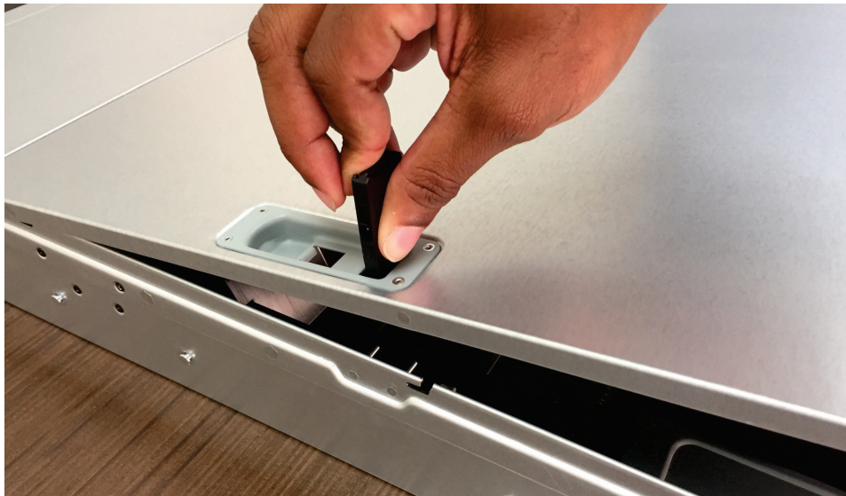
Figure 55. Replacing the 2145-SV1 back cover
