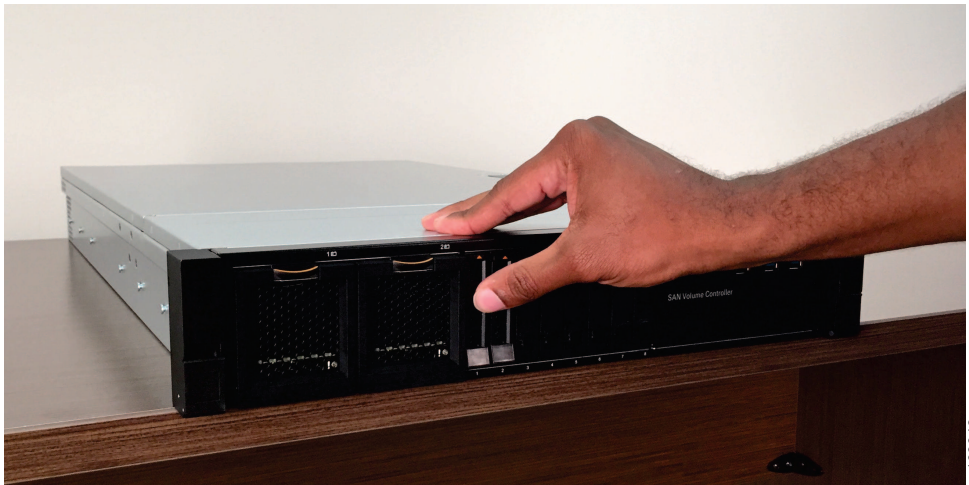
Figure 87. Closing the release handle on a 2145-SV1 boot drive
