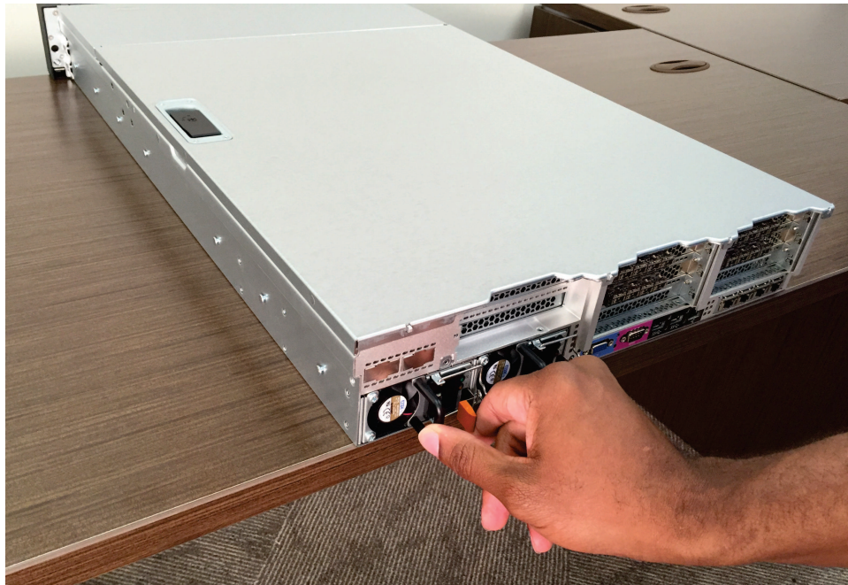
Figure 137. Removing the 2145-SV1 power supply
