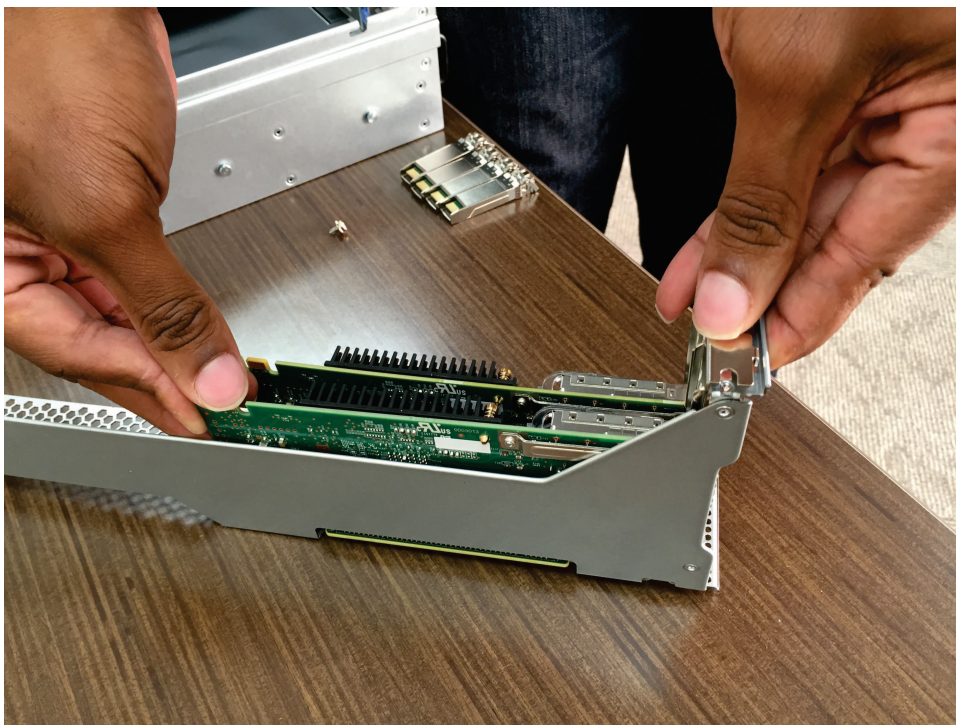
Figure 158. Aligning the adapter into the PCI connector
