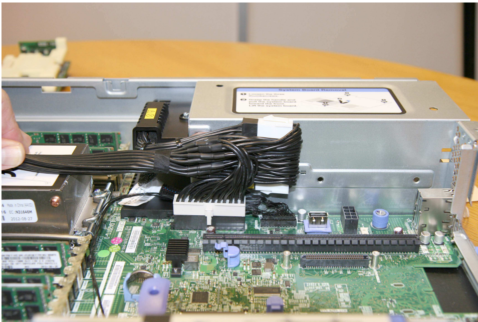
Figure 116. Power cable connection between the power supply unit and the system board
