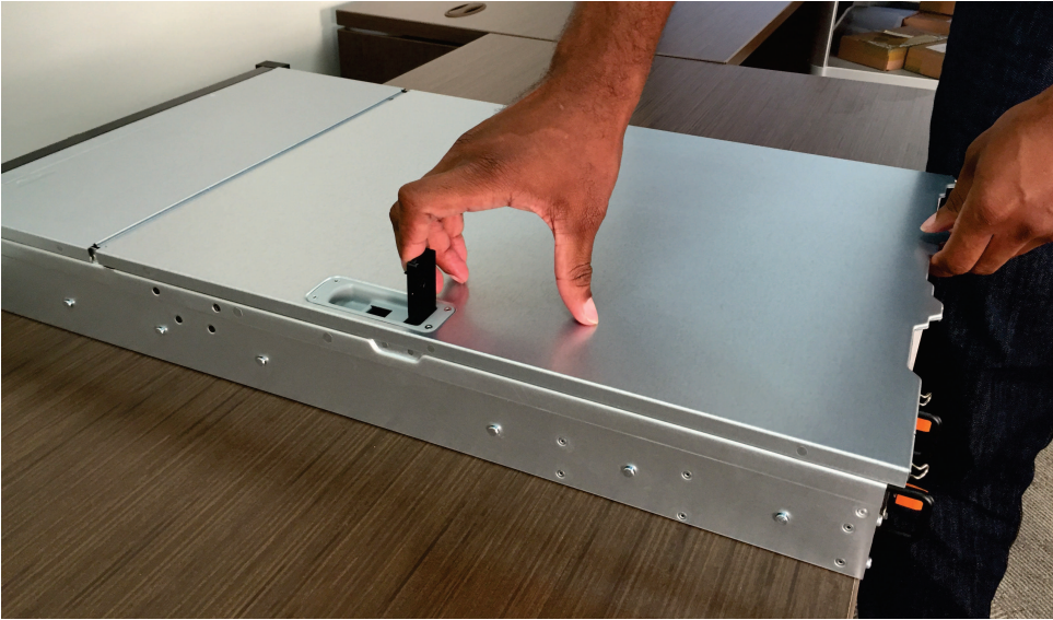
Figure 50. 2145-SV1 back cover release latch
