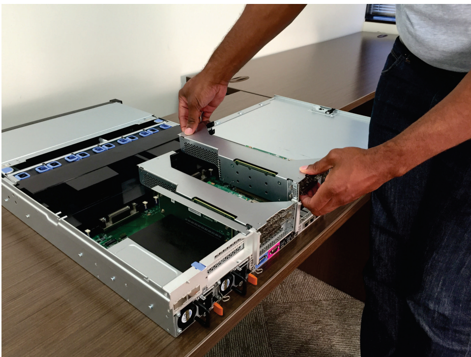
Figure 147. Removing PCI riser card assembly 1
