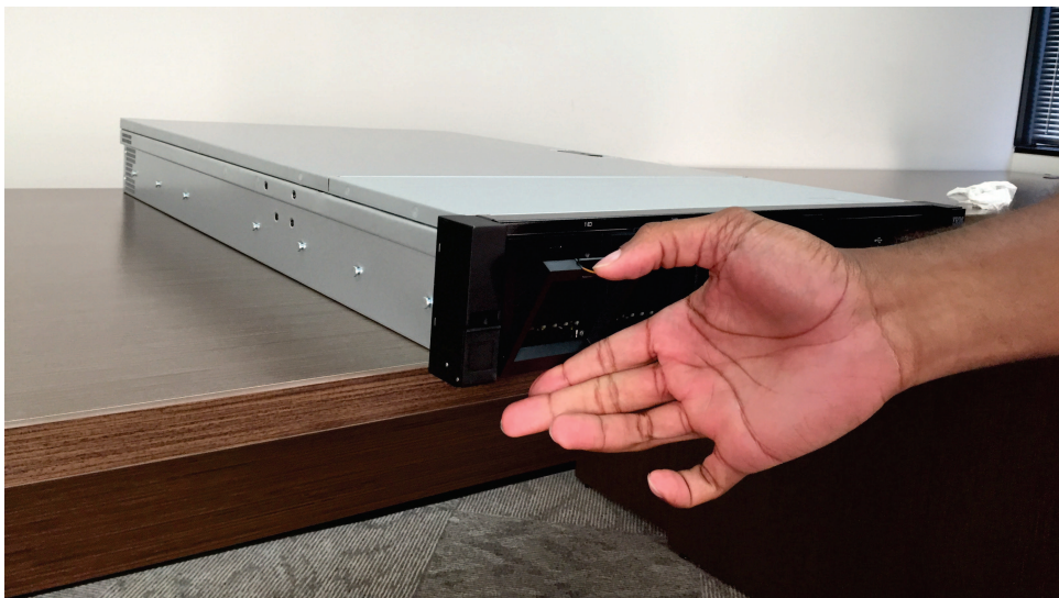
Figure 121. Release the battery module on the 2145-SV1 node
