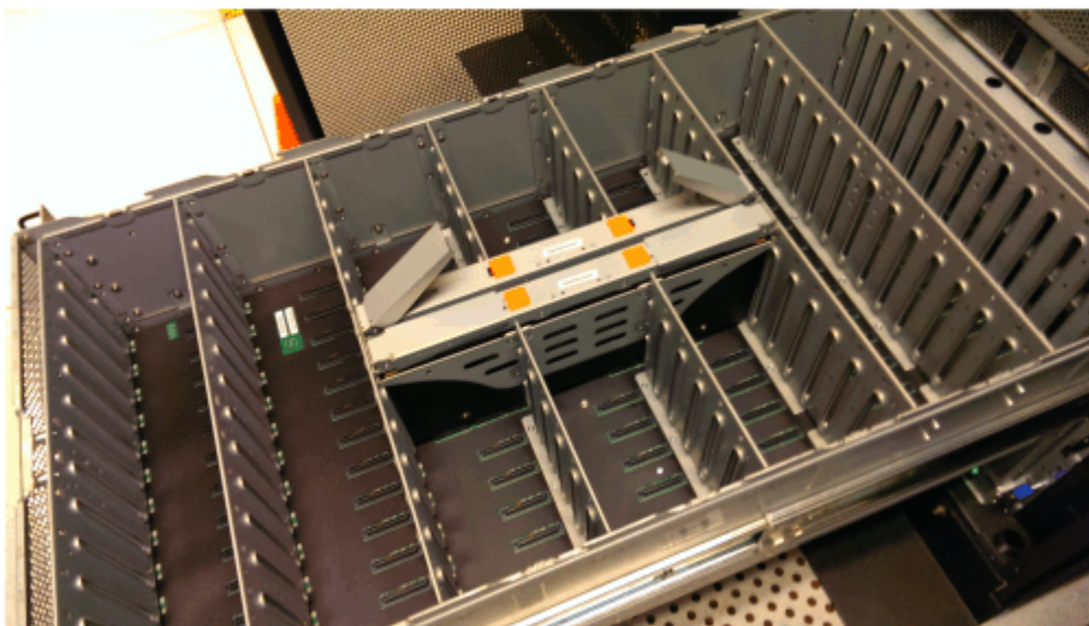
Figure 113. Location of secondary expander modules
