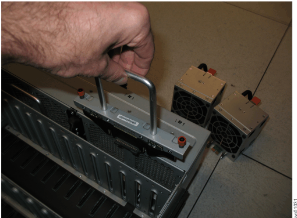
Figure 126. Remove the FIB from the chassis
