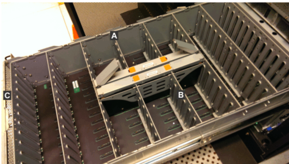
Figure 86. Location of secondary expander modules
