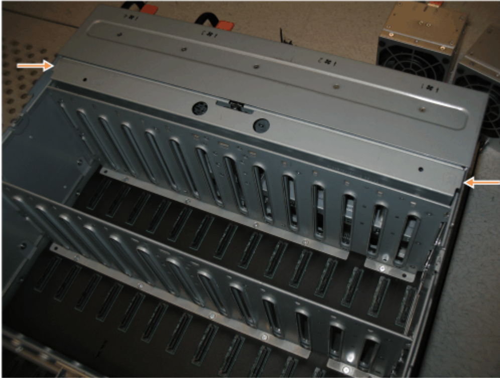
Figure 106. Replace the FIB cover
