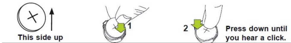
Figure 20. Install the battery
