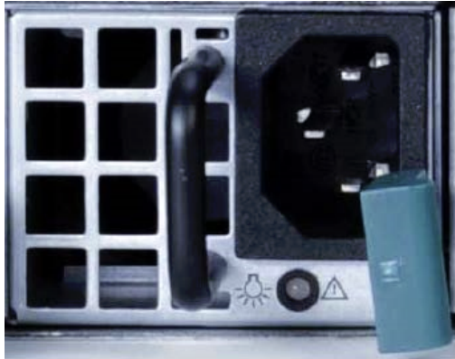
Figure 18. Removing a PSU from the chassis
