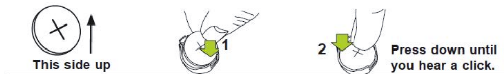
Figure 32. Install the battery
