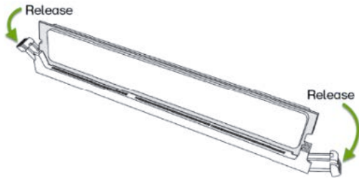
Figure 23. Releasing a memory module from its slot
