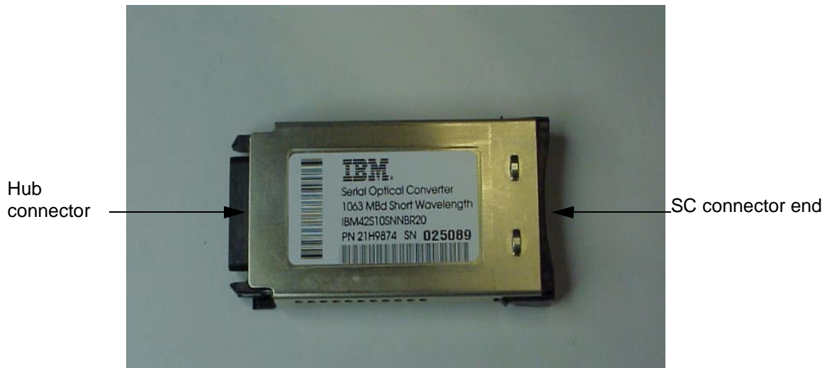
Figure 2. SWL fiber-optic GBIC (part number and labeling varies)
