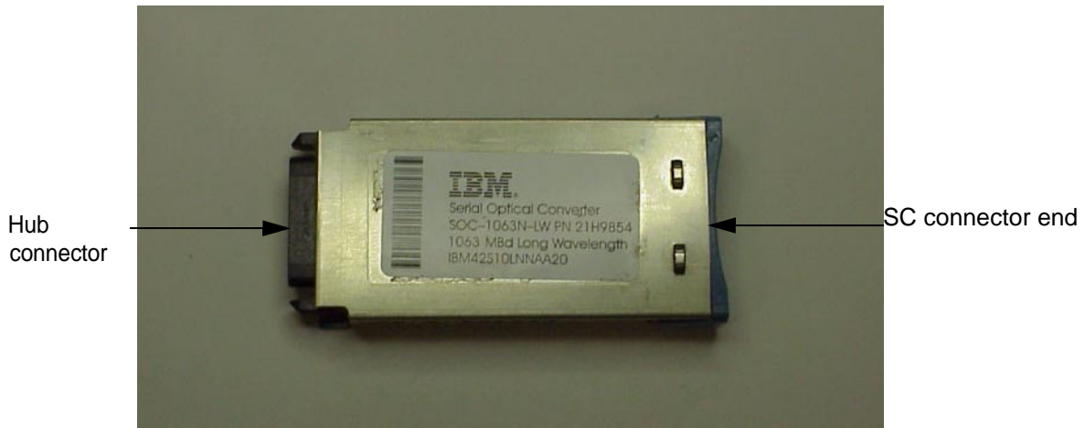
Figure 3. LWL fiber-optic GBIC module (part number and labeling varies)
