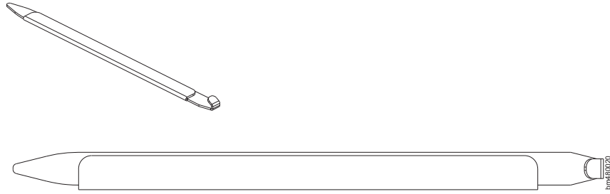
Figure 37. Optical transceiver (SFP+) extraction tool
