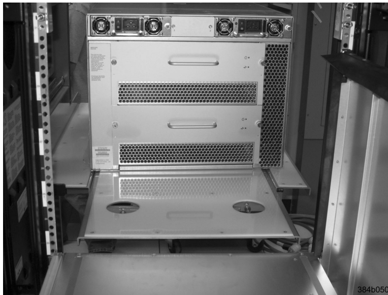
Figure 12. Load plate extended inside the cabinet to the exhaust kit shelf
