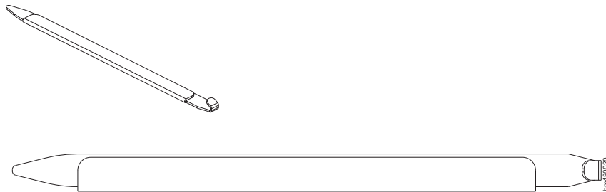
Figure 42. Optical transceiver (SFP+) extraction tool
