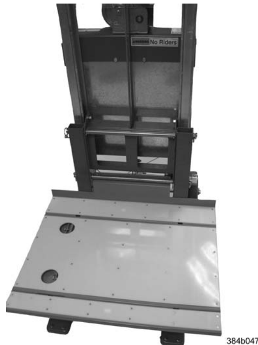
Figure 4. Assembled lift tool with 24-inch load plate
