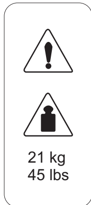
Figure 14. Weight label on battery unit of uninterruptible power supply
