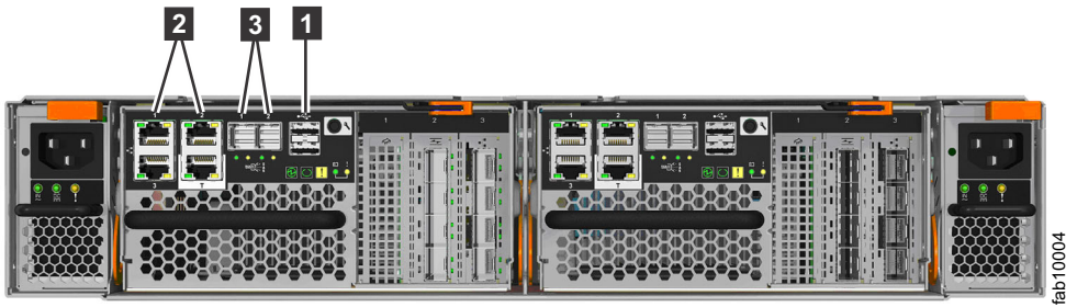
Figure 19. Storwize V7000 2076-524 node canister ports
