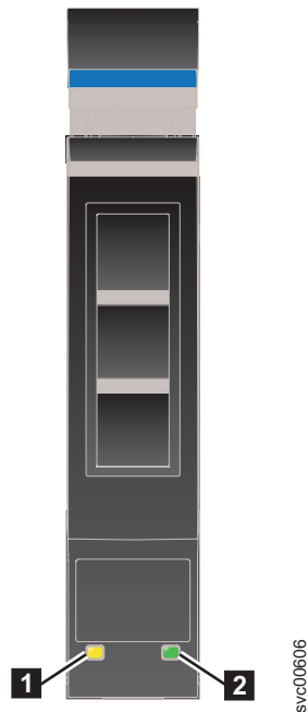
Figure 9. LED indicators on a single 2.5" drive
