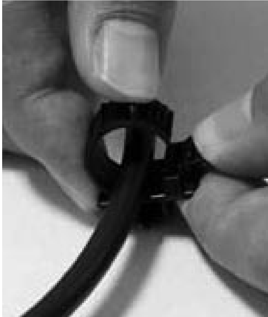
Figure 55. Unlocking the cable retention bracket
