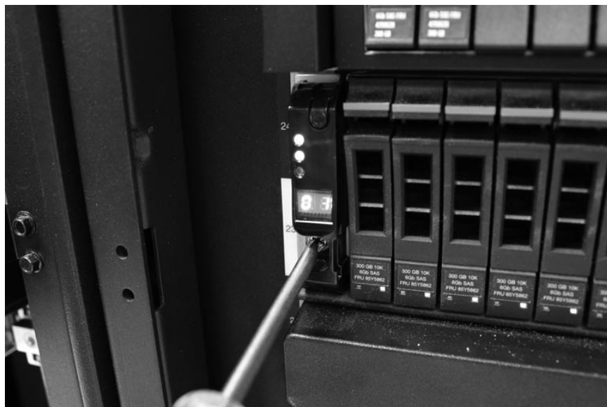
Figure 23. Securing an enclosure to a rack cabinet
