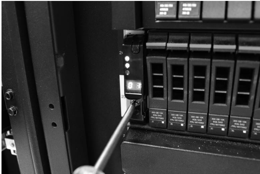
Figure 19. Securing an enclosure to a rack cabinet
