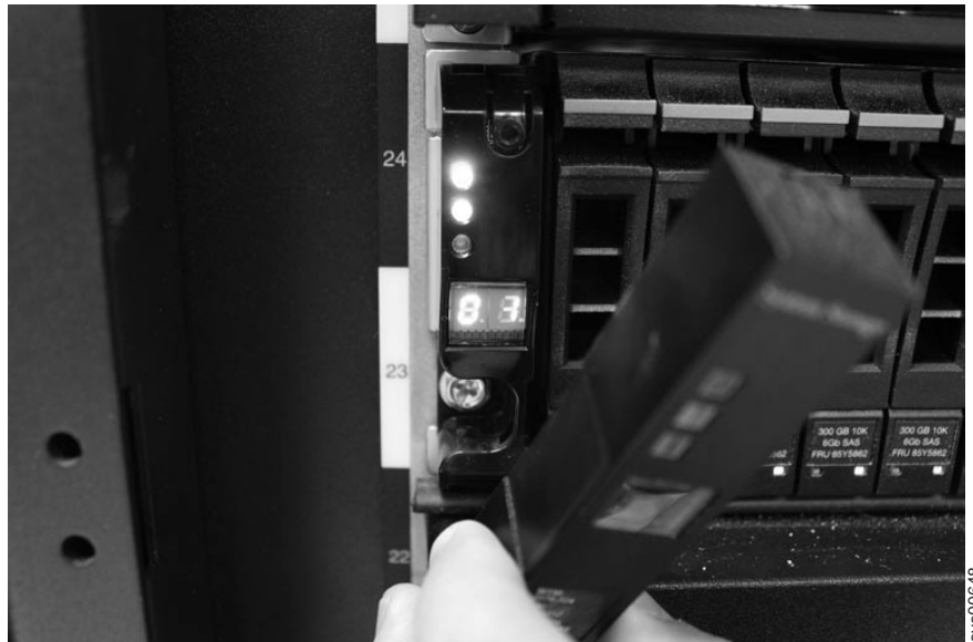
Figure 22. Removing the enclosure end cap
