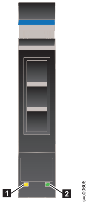
Figure 11. LED indicators on a single 2.5 inch drive
