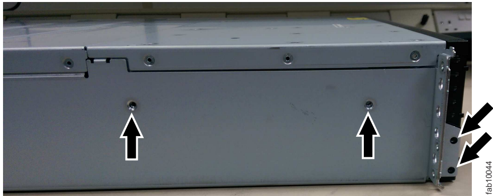
Figure 106. Left-side enclosure screws
