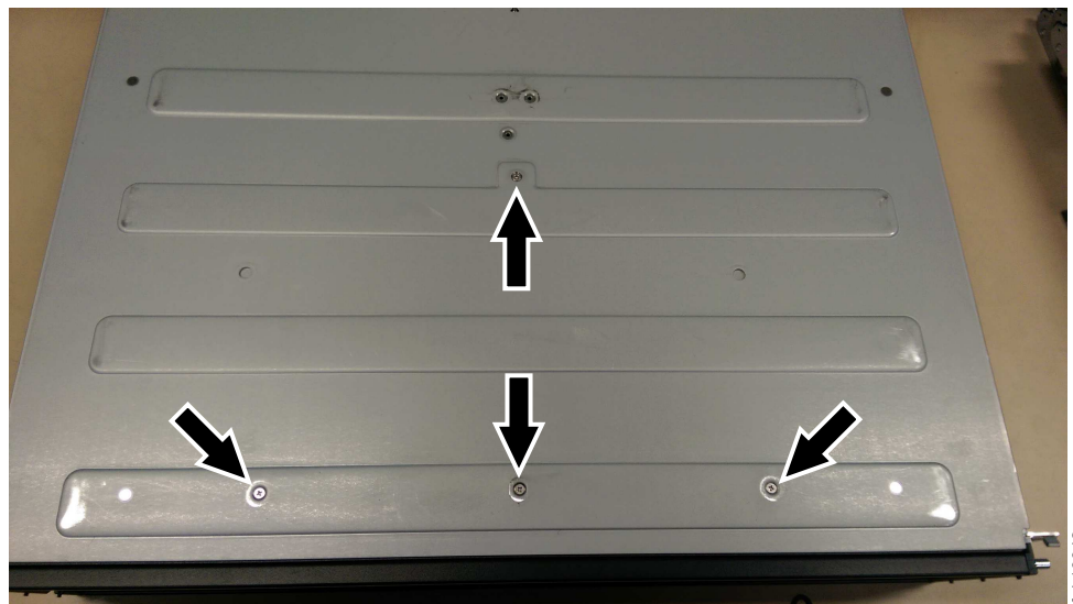
Figure 104. Bottom enclosure screws
