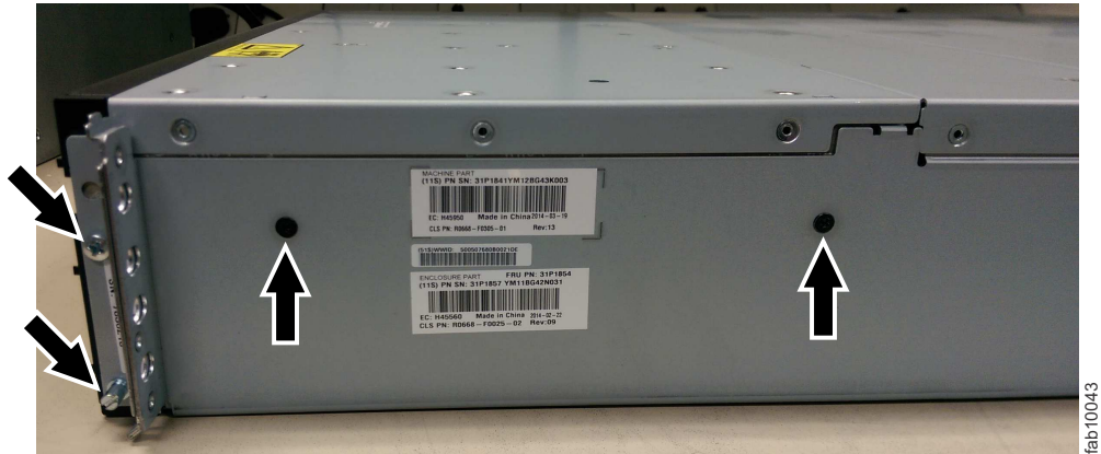
Figure 105. Right-side enclosure screws
