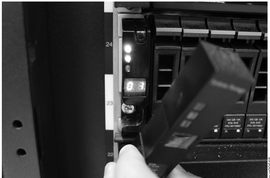
Figure 22. Removing the enclosure end cap
