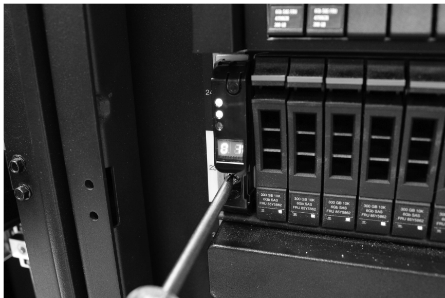
Figure 23. Securing an enclosure to a rack cabinet
