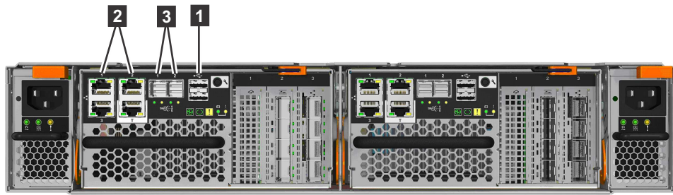
Figure 7. Data ports in the rear of the Storwize V7000 Gen2 control enclosure (2076-524)
