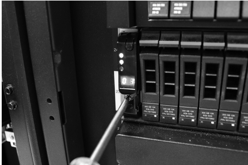
Figure 19. Securing an enclosure to a rack cabinet
