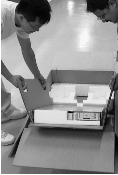
Figure 144. Slide the 2145 UPS to the edge of the carton
