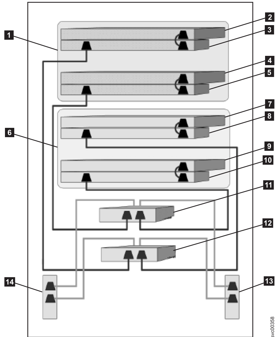
Figure 1. A four-node SAN Volume Controller cluster with the redundant ac power switch feature
