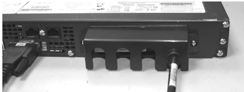
Figure 18. 2145 UPS-1U power cable-retention bracket
