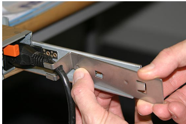
Figure 80. Attaching the cable retention bracket to the SAN Volume Controller 2145-8F4 power cable
