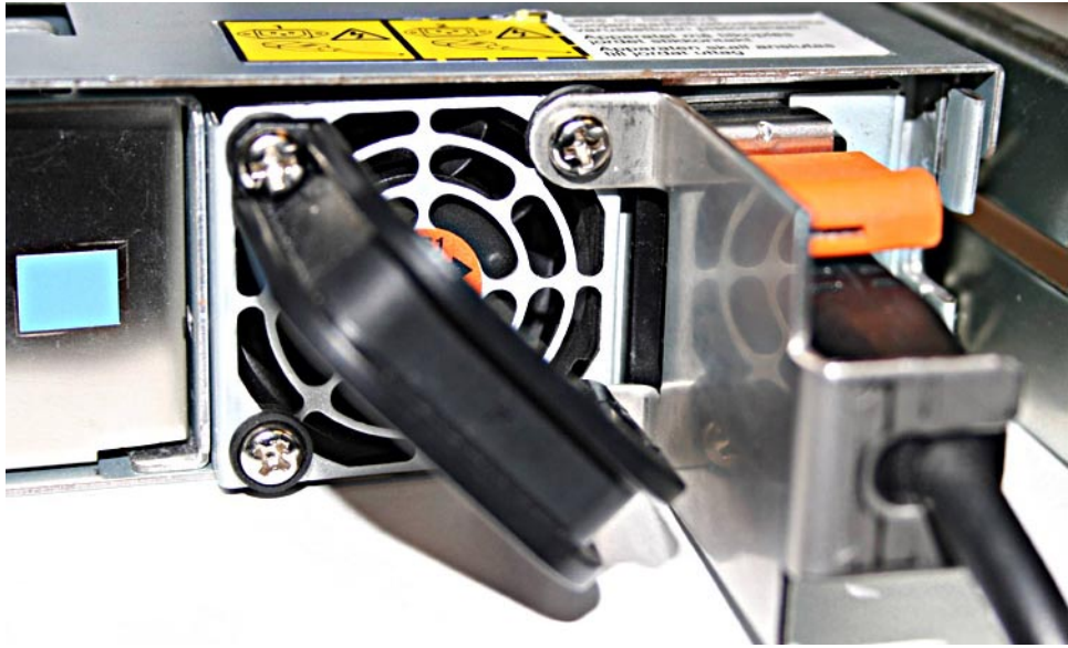
Figure 42. The SAN Volume Controller 2145-8G4 with the cable retention bracket attached
