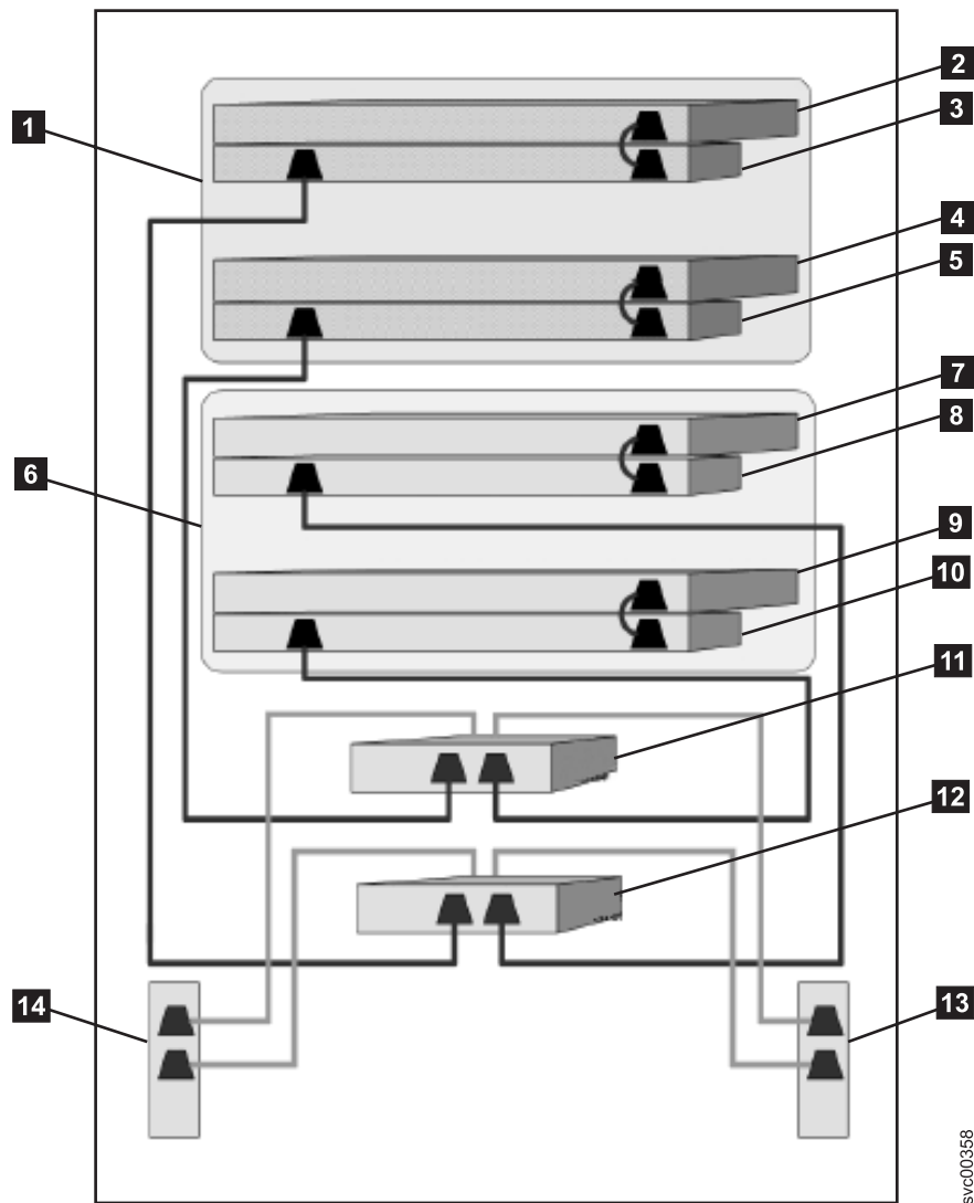
Figure 4. A four-node SAN Volume Controller cluster with the redundant ac power switch feature
