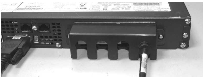
Figure 19. 2145 UPS-1U power cable-retention bracket
