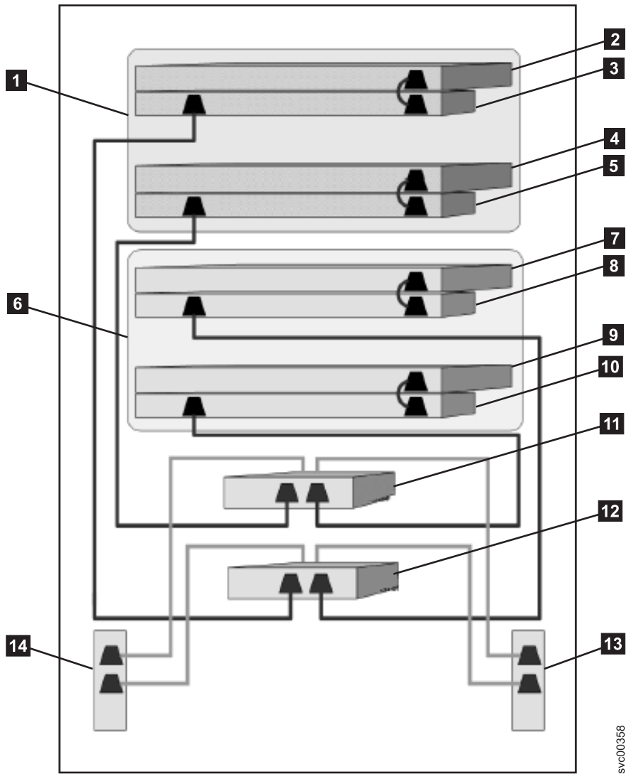
Figure 2. A four-node SAN Volume Controller cluster with the redundant ac-power switch feature
