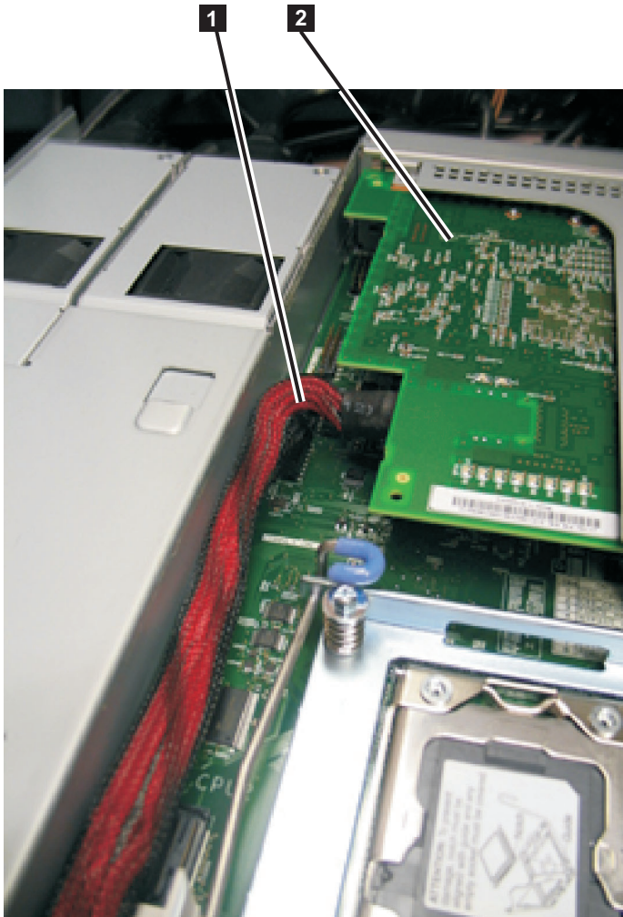
Figure 192. High-speed SAS adapter assembly and high-speed SAS cable in the SAN Volume Controller 2145-CF8
