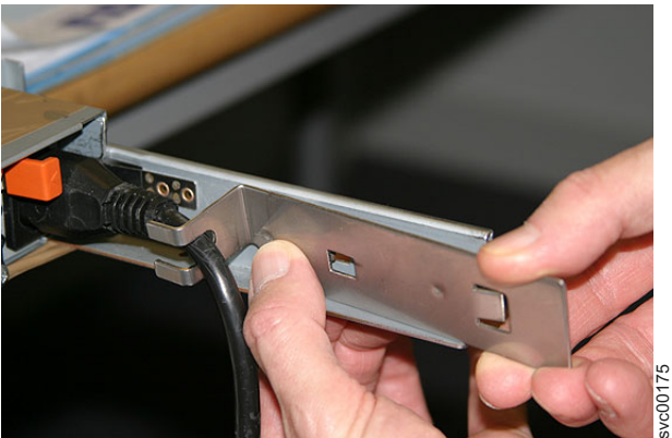
Figure 36. Attaching the cable retention bracket to the SAN Volume Controller 2145-8F4 power cable
