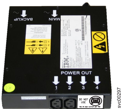
Figure 1. Photo of the redundant ac-power switch
