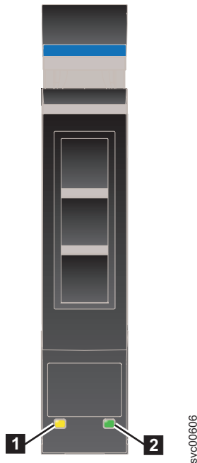
Figure 4. LED indicators on a single 2.5" drive
